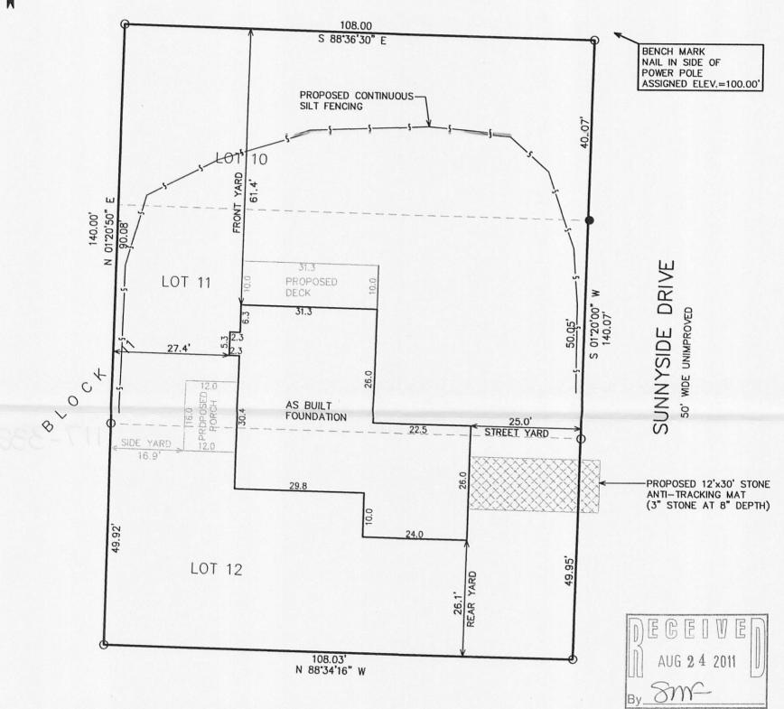
LOWEST GROUND ELEVATION AT BUILDING FOOTPRINT=100.8' PLUS 35' MAXIMUM BUILDING HEIGHT MAXIMUM ROOF PEAK ELEVATION=135.8'
